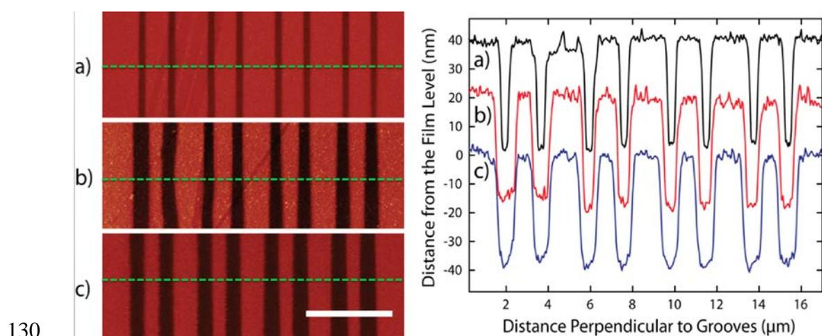
131 **Figure 3.** AFM images of structures written with  $I_{dlw}$  of (a)  $80 \text{ GW/m}^2,$  (b)  $240 \text{ GW/m}^2$  and
