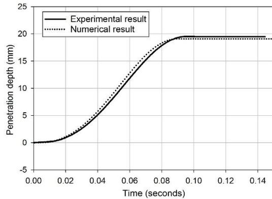
Fig. 7. Validation of the penetration depth vs. time.
