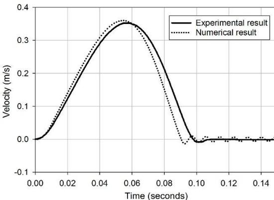
Fig. 8. Validation of the penetration velocity vs. time.
