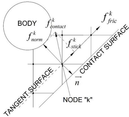
Fig. 3. Clay body – cone contact interaction.
