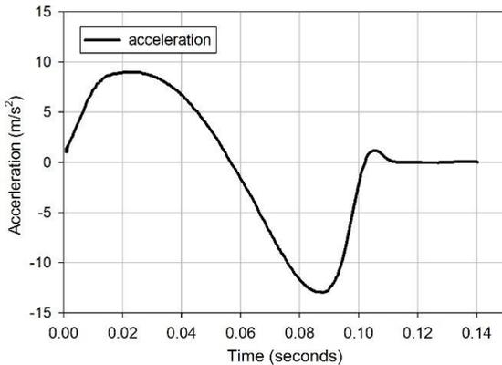
Fig. 6. Acceleration measurement during the penetration [7].
