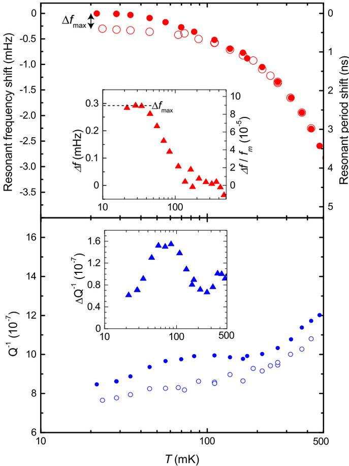
**Fig. 2** Temperature dependence of the TO resonant frequency (*top*) and inverse quality factor (*bottom*). In both plots, open symbols show measurements for the empty cell and closed symbols are for measurements with a polycrystalline sample of solid  $^4\text{He}$ . The frequency shift is shown with respect to the low temperature value. The *insets* show the corresponding shifts due to solid helium after the empty cell data has been subtracted (Color figure online)
