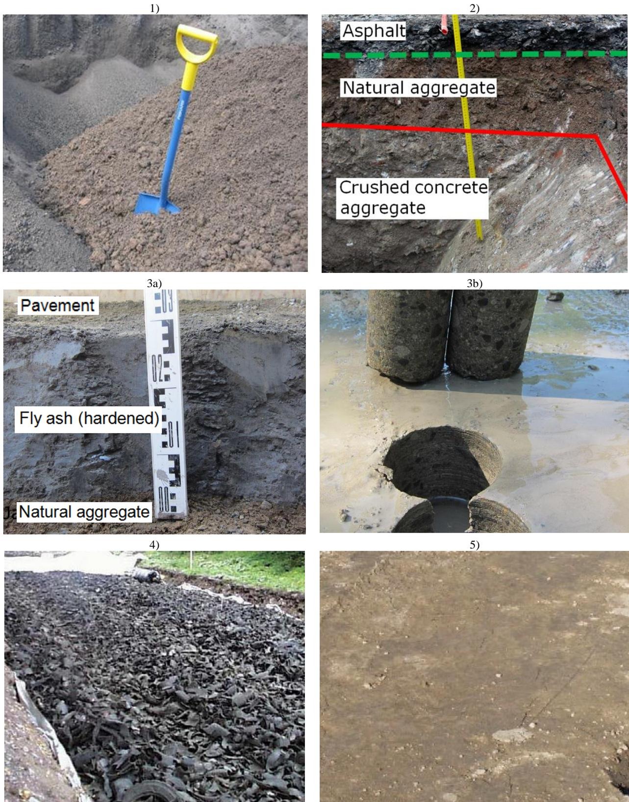
Figure 4 Figures of UUMA-material types 1-5: 1) Bottom ash ([www.uuma2.fi](http://www.uuma2.fi)); 2) Crushed concrete, re-hardened (Dettenborn et al. 2016); 3a) Cement stabilised fly ash; 3b) Fly ash stabilised crushed aggregate (Tarkkio 2014); 4) Shredded tires as a light weight material of street embankment (Forsman et al. 2002); 5) Stabilised surplus clay as a liner (Forsman & Leivo 2007). The explanations for the material types 1-5 are presented in Table 1.
